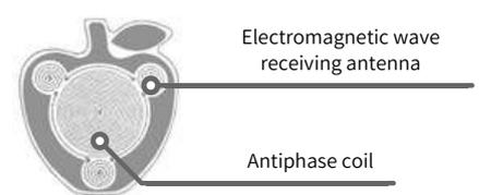
Absorb radio waves and electromagnetic waves from the antenna and create zero magnetic field by flowing current in the coil.
